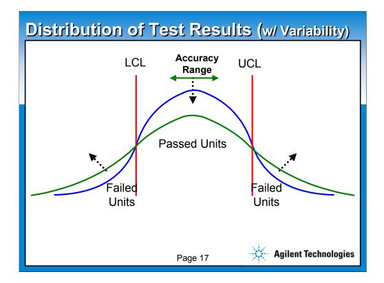
When the test solution used in the test has variability and is not accurate the distribution of the test results is flatter, spread out more and shifted off of the absolute accuracy point. This could causes units on the fringe of the limits to fail falsely, an NTF, or to pass falsely, an escape. NTFs cause the cost of test increase. Escapes can also cause a higher cost of test, but more damage is done to the reputation of a company when an escape makes it into the customer's hand.
