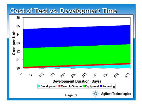
I just briefly want to touch on the impact the time it takes to develop a test process has on the overall cost per unit. As you can see from the graph, unless the development time is changed drastically, like by a 200 days, development time has little impact on the per unit cost.
