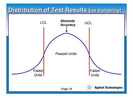
In this graph the results of a test is a normal gaussian curve. The red lines signify the lower and upper limits of the tests. Units that measure between these limits pass and those outside the limits fail. With the test solution having no variability and absolute accuracy, the distribution will solely be based upon the variability of the units tested.
