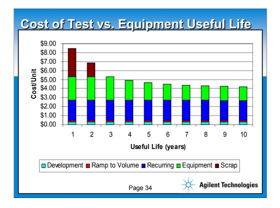
So the model is loaded and we are now looking at the results of the sensitivity analysis. This first graph highlights the cost of test versus the useful life of the equipment.
