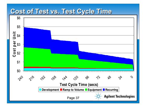
This slide highlights the impact test time has on the cost of test.
