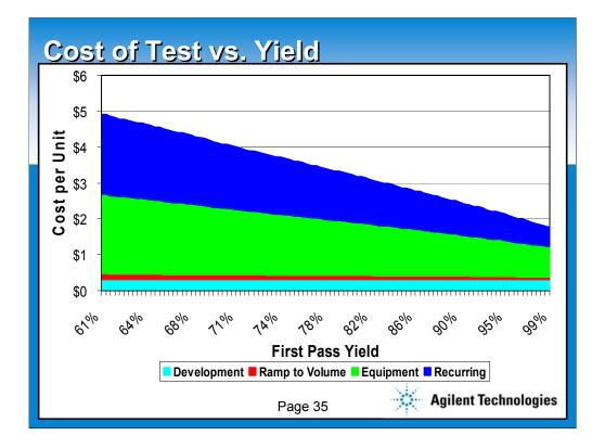
Okay we made it through the most difficult graph. This graph highlights the impact yield has on the cost of test. This graph is a stacked area graph. Meaning the incremental change in the different elements is added to the previous elements until the top of the entire colored area represents the cost of test per unit produced.
